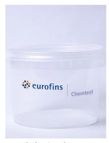
**500ml plastic tub**Uses: asbestos and inorganics e.g., metals, BRE, cyanide
